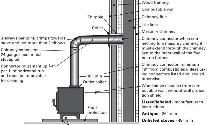
**Floor protection for all stoves** must extend at least 18" beyond the stove / insert on all sides, be noncombustible, and installed according to manufacturer's instructions.
